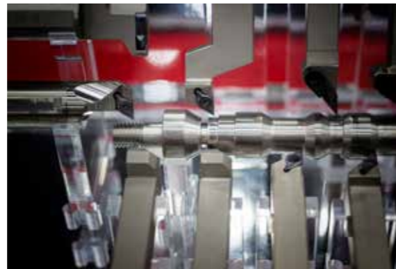
Figure 1 – A typical turning operation on a powertrain component.
