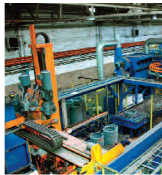
Blasting station for rings.
