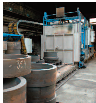
Furnaces for heat treatment of rings.
